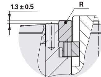
**Front-end shaft coupling (with mechanical fault exclusion)**
