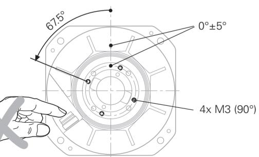
Changed 0° position and mounting holes compared with RCN 22x.
