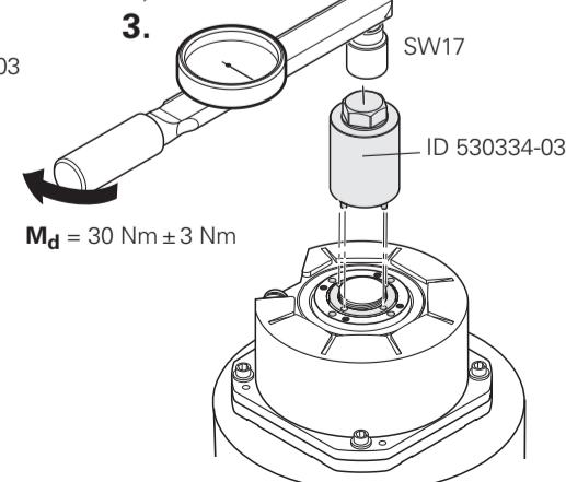
**Front-end shaft coupling (without mechanical fault exclusion)**
