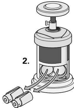
Included in the delivery: 2 Alkaline batteries, 1.5 V, LR1
