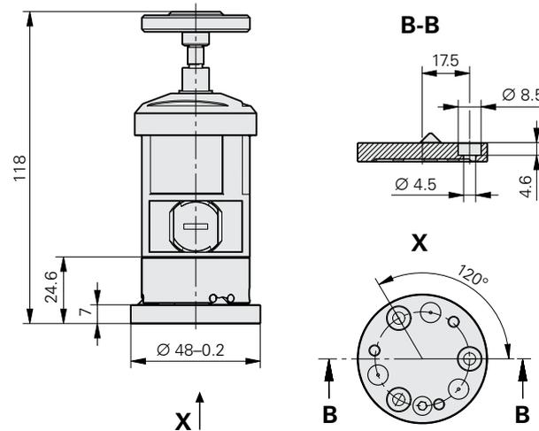
**Mounting the probe contact**
