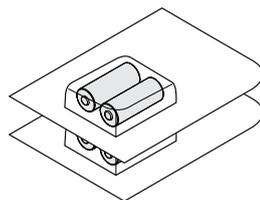
2x 2 alkaline batteries, 1.5 V LR1
