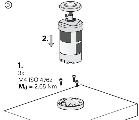
**Exchanging the connection pin / probe contact**
