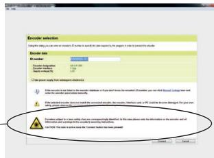
Encoders subject to a laser safety class are correspondingly identified. In this case please note the information on the encoder and all information and warnings in the encoder's mounting instructions.
