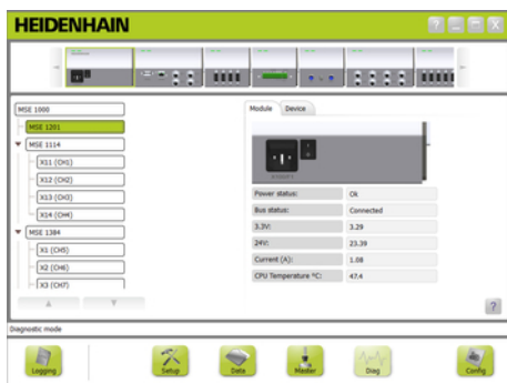
Power supply module diagnostics screen
