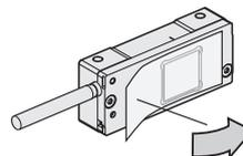
If necessary: Clean the graduation of the scale tape and scanning head
