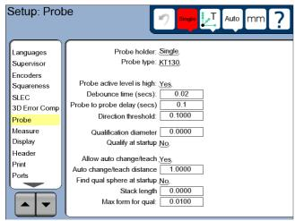
Probe setup page with Max form for qual parameter
