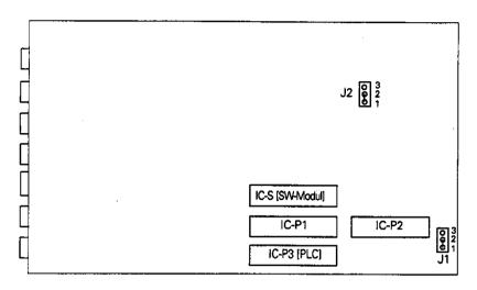
The NC software is located in sockets IC P1 and IC P2 (two 4-MB EPROMs)
