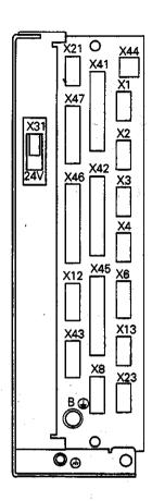
X1 = Measuring system 1 (~) X2 = Measuring system 2 (~) X3 = Measuring system 3 (~) X4 = Measuring system 4 (~) X6 = Measuring system S ( □ ) X8 = Nominal value outputs 1,2,3,4,S X12 = Touch probe system 1 X13 = Touch probe system 2 X21 = Data interface RS-232-C/V.24 X23 = Handwheel HR130 X41 = PLC output X42 = PLC input X43 ≠ VDU X45 = TNC keyboard X46 = Machine operating panel X47 = PLC I/O board PL 410B Power supply 24 V for NC X44 = Power supply 24 V for PLC = Signal ground
