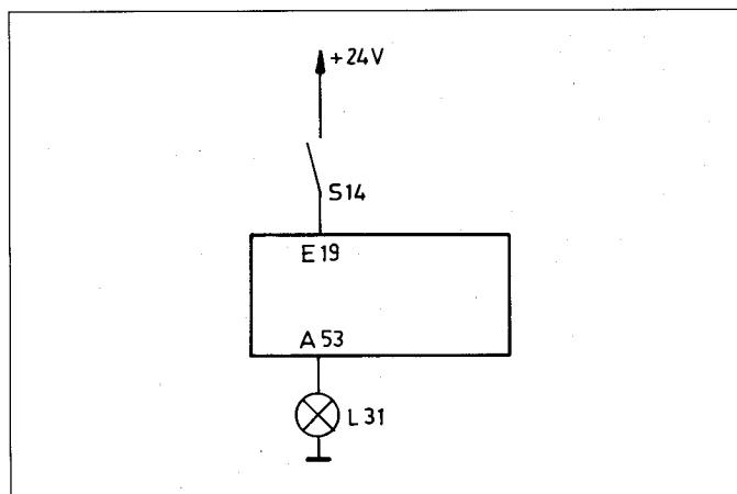
Lamp 31 should illuminate in the event of contact S14 being open.
