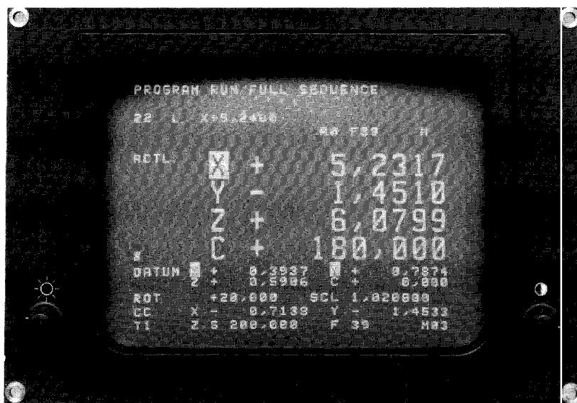
The NC-part of the control signals a program interruption to the PLC via marker 2183 (display flashes). The initial status is signalled via the marker 2184 (display on or flashing). When both markers are reset, the program run has been terminated.
