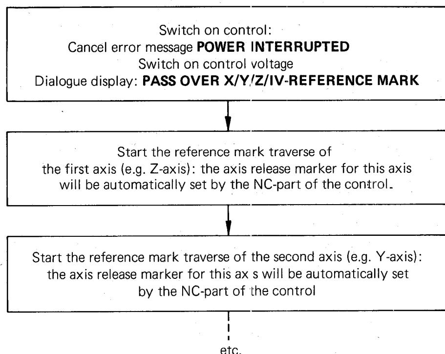
The axis release markers remain set to "1" after traversing over the reference marks, thus keeping the machine axes in closed positioning loop through the control.
