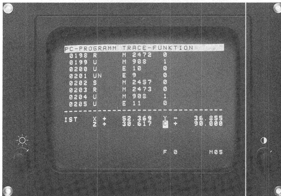
In this mode, the function of the PLC-program can be checked in the RAM-memory. In addition to the PLC-commands, the logic state of the operands and gating results are displayed. The logical status of a marker at input or output is displayed additionally before display of the gating result.
