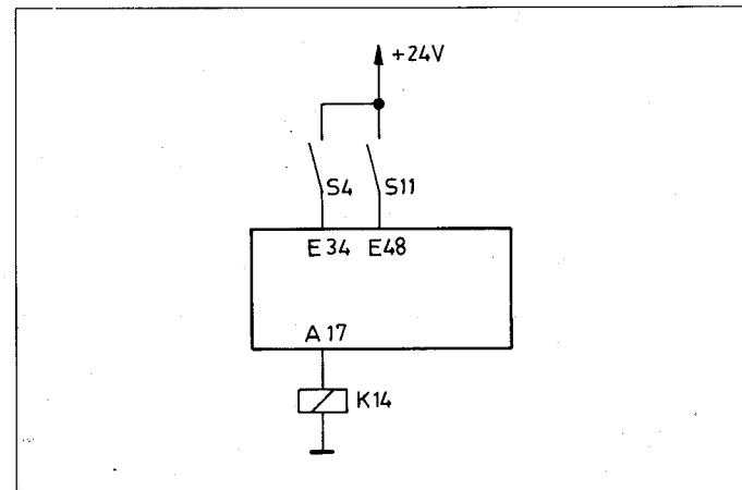
The relay K14 should energise when contact S4 or S11, or both, are open.
