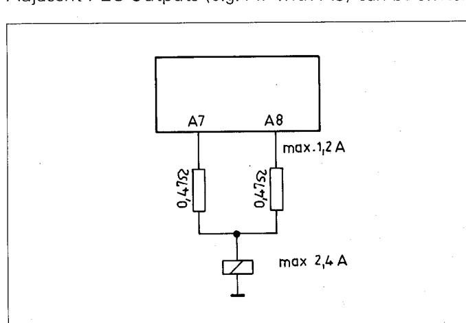
**Bipolar outputs** (PL 110 B; A25 to A30 and A57 to A62)
