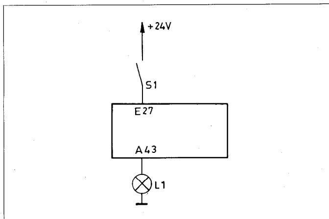
The lamp L1 is connected to the output 43. The closing of the contacts S1 should result in the illumination of the lamp. The contacts are connected to input E27 of the PLC.
