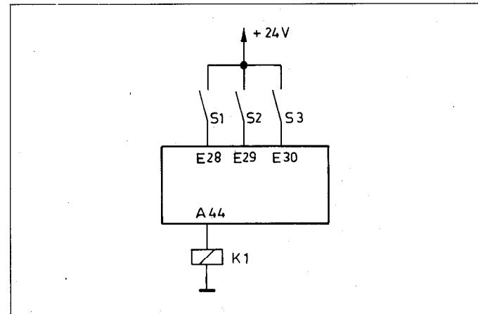
The relay K1 should energise, in the event of the contacts S1, S2 and S3 closing simultaneously.
