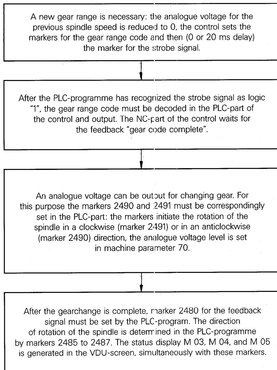
After the gearchange is complete, the control outputs the relevant analogue voltage (determined by machine parameters 86, 87, 88, 89).
