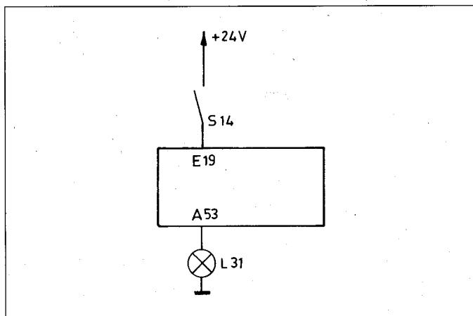
The lamp L31 should illuminate when the contact S14 is opened.
