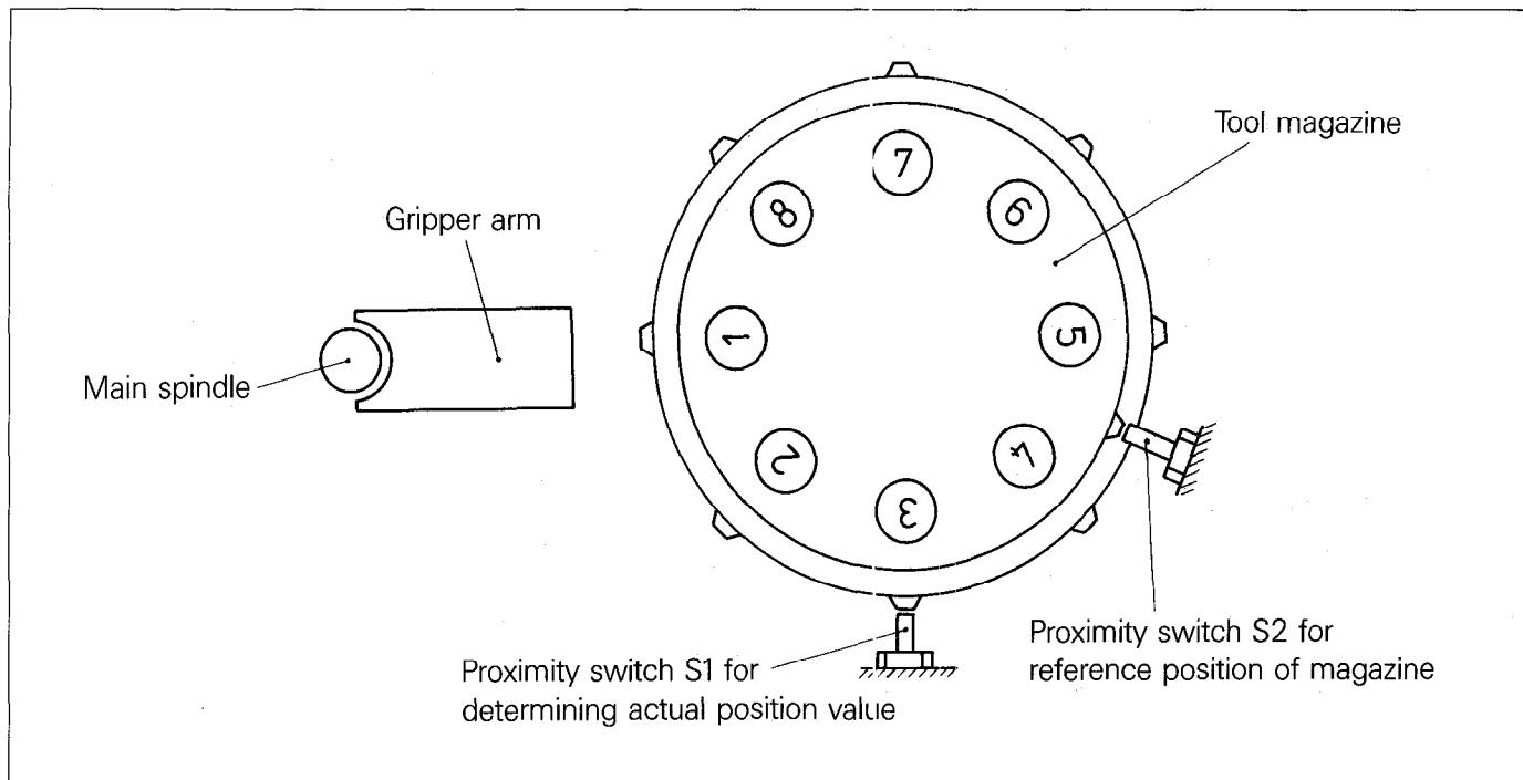
.With the first tool call, the tool magazine is rotated to the reference position (proximity switch S2). On reaching the proximity switch, the markers for the actual value of the pocket number (M 3032 to M 3039) is set.
