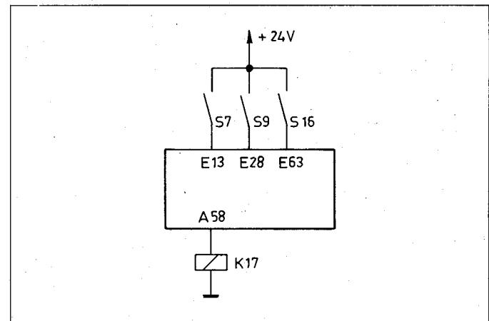
The relay K17 should only energise when all three contacts S7, S9 and S16 are open.
